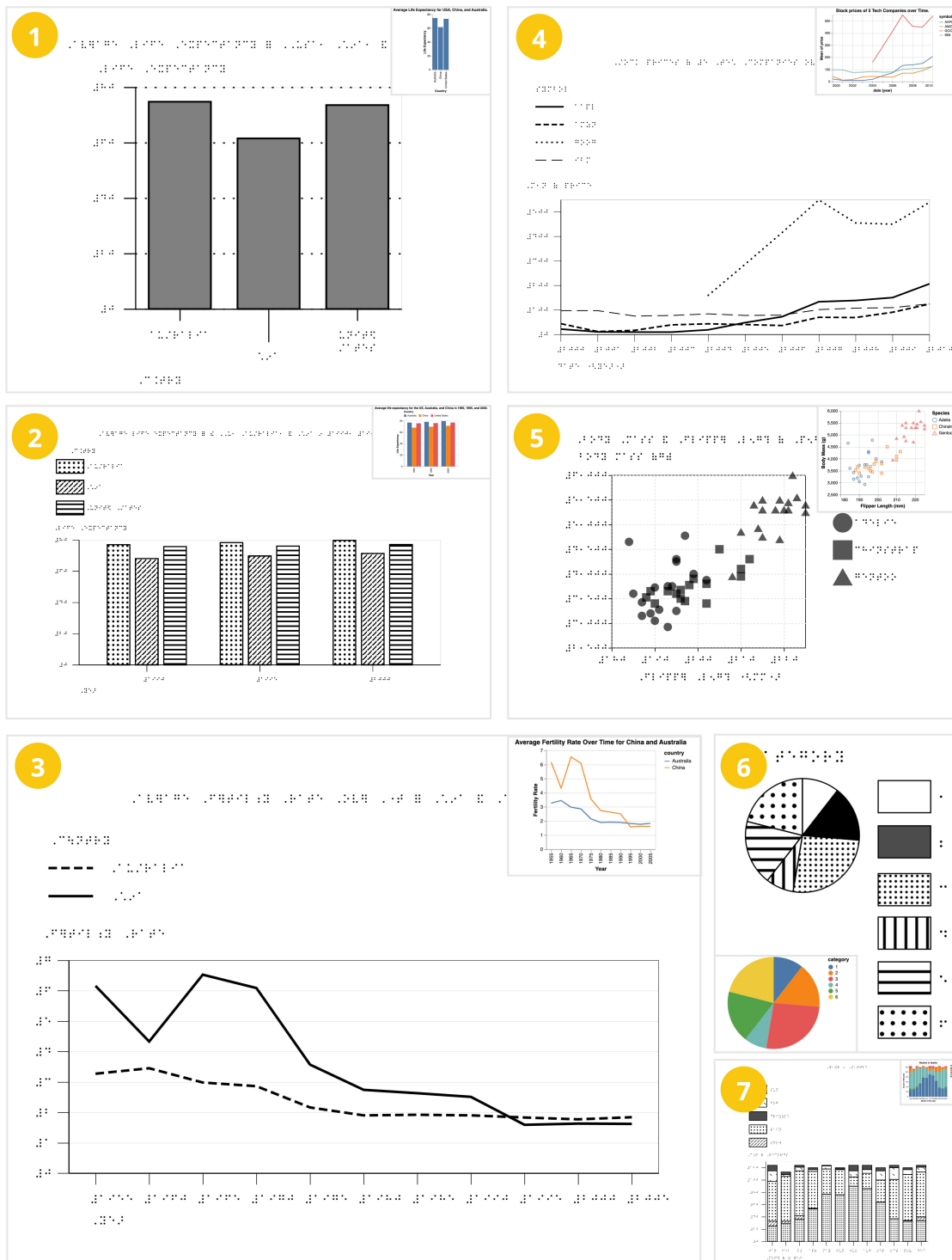
Figure 8: Gallery of tactile chart examples demonstrating various chart types, including bar charts, line charts, scatter plots, pie charts, and stacked bar charts. Each tactile chart is accompanied by its visual counterpart, showcasing how texture-based encodings, braille annotations, and tactile legends make data tactually accessible.
