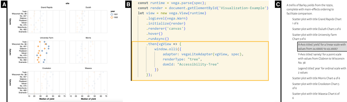
Figure 1: A) An example visualization. B) Example Olli code using a Vega-Lite adapter. C) An accessible tree view rendered by Olli.
